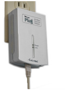
An example of a powerline Ethernet adapter
